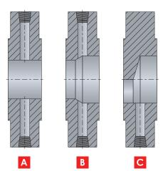
Our flush ring design is made to accept all flanged pressure transmitters on one side and a standard ANSI flange on the other side in all sizes.
